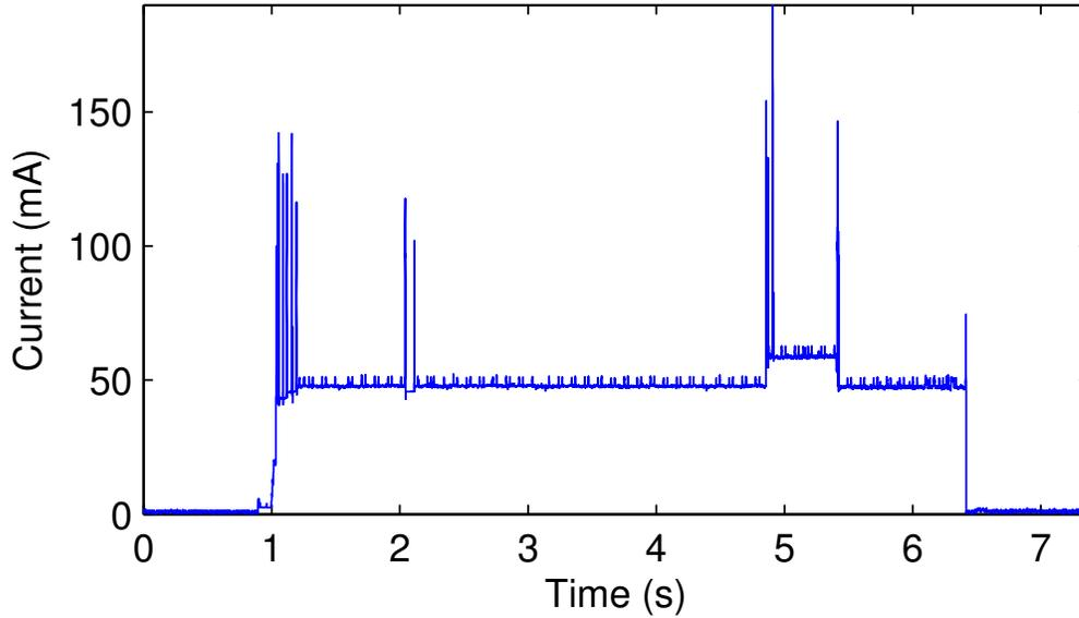
Figure 4.15: Current consumption during transmission of stored measurement data. In this example,  $75 \mu\text{Ah}$  was drained from the battery (excluding standby current).
