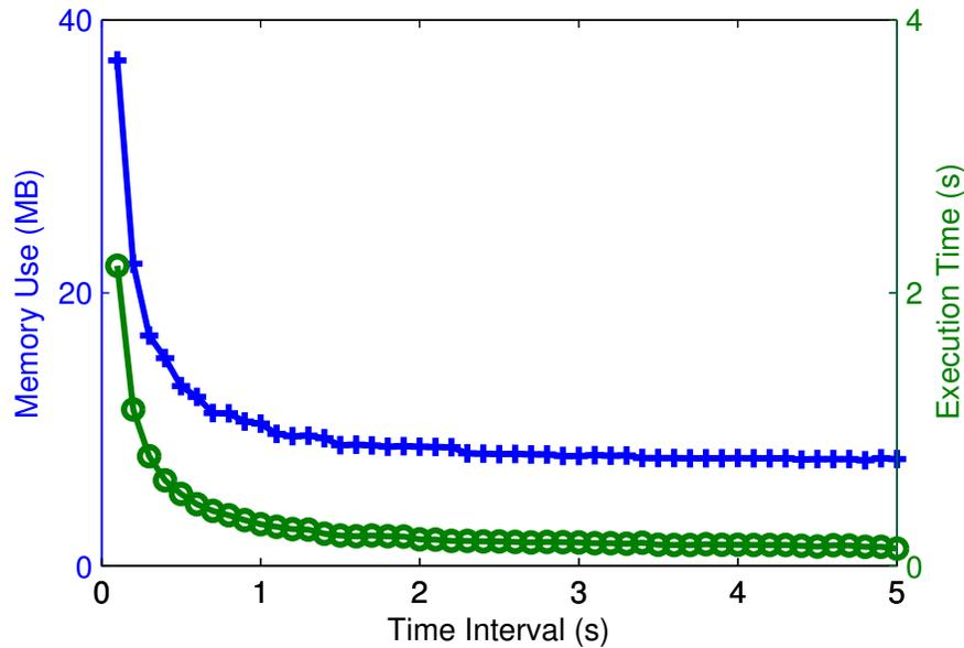
Figure 6.15: Plot of the resources used as a function of the time interval,  $\delta t$ . Memory usage given by + markers and execution time given by o markers.
