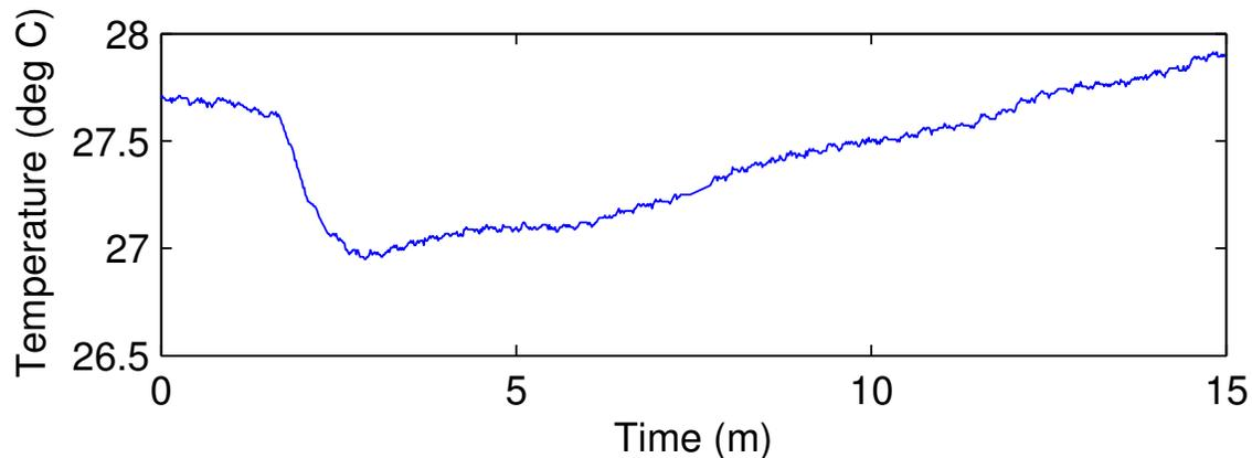
Figure 6.20: Cooling effect induced by walking. Between minute 1 and minute 3, the occupant is walking from the desk to the lab location. After minute 3, the occupant is seated at the lab location
