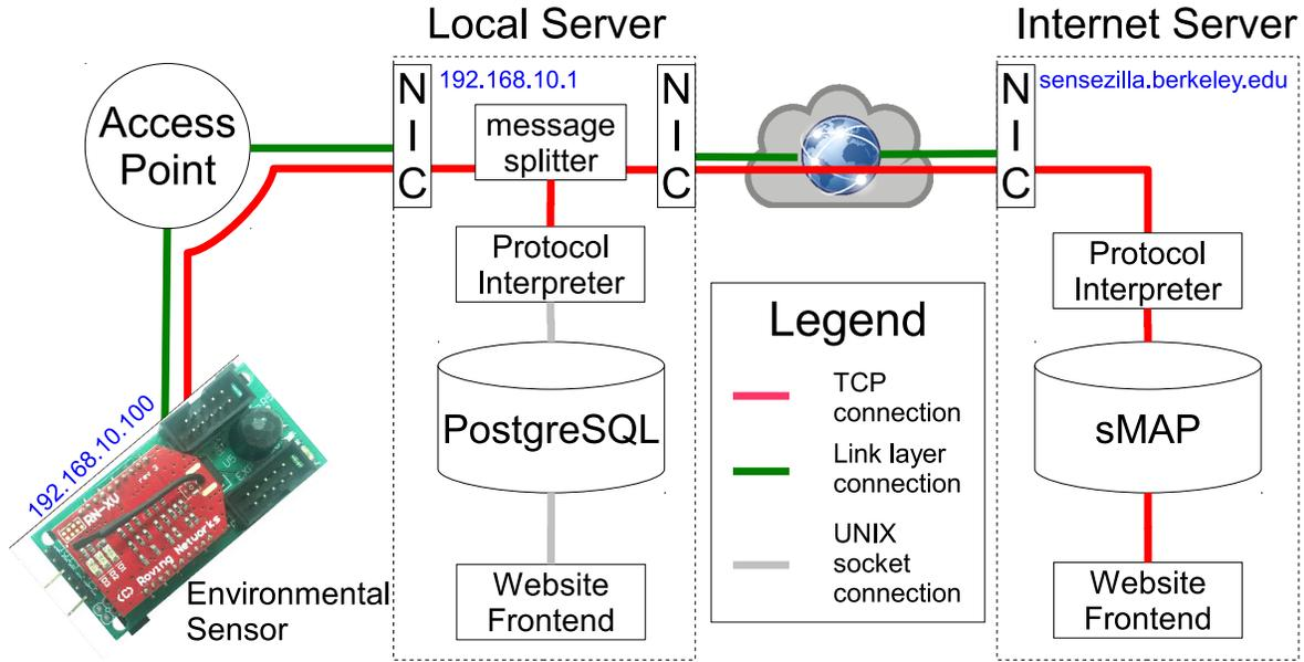
Figure 4.1: Network diagram showing the connections made during normal operation. The TCP connection from the sensor to the local server is only active while the sensor is transmitting a report.
