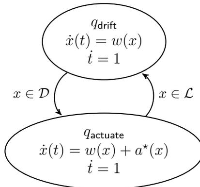
Figure 3.6: On-board controller hybrid automaton diagram.
