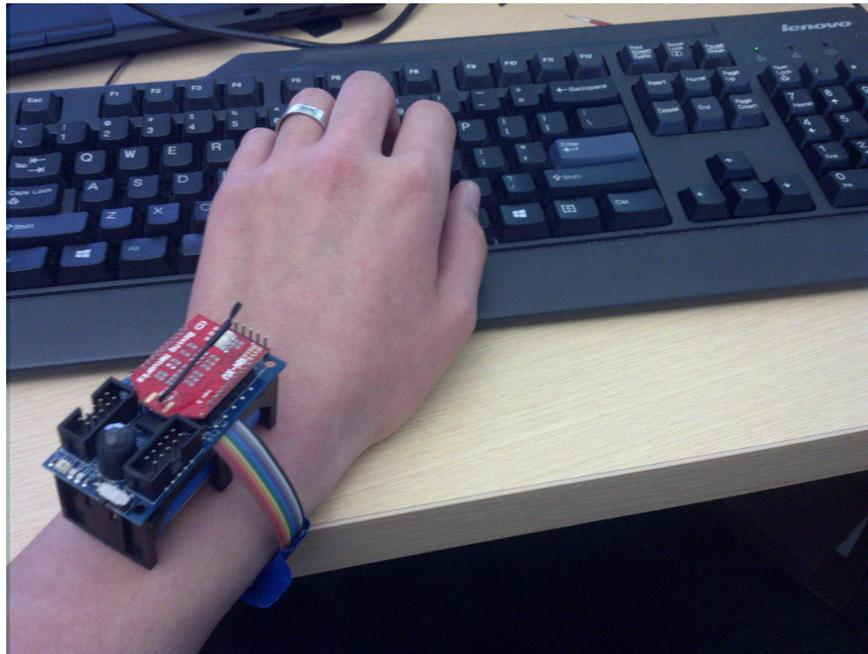
Figure 6.18: Occupant-carried environmental sensing watch
