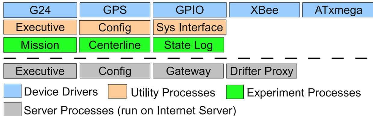
Figure 2.9: Set of Python modules (processes) running during a typical experiment.
