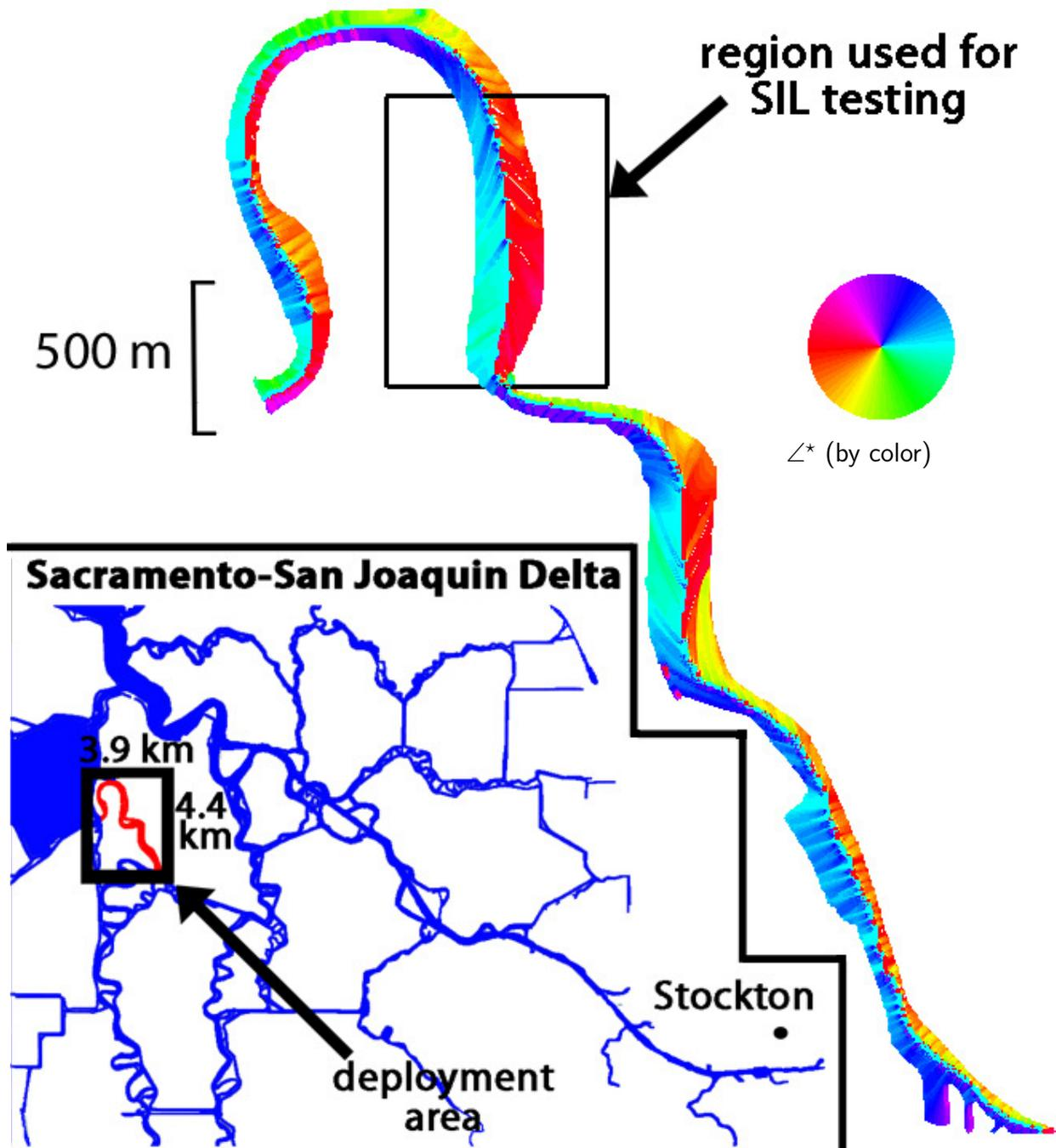
Figure 3.4: The optimal bearing to center of the river,  $\angle^*(x)$ .
