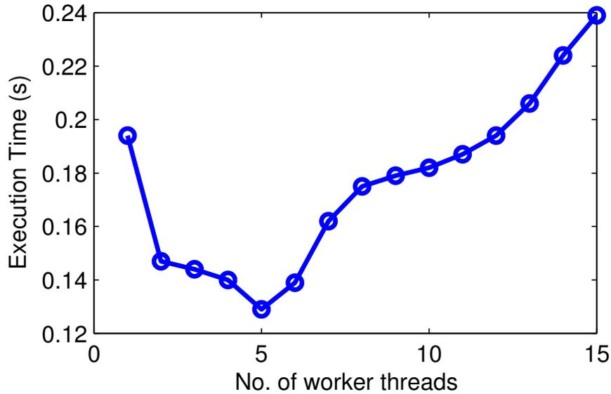
Figure 6.16: Plot of execution time as a function of the number of the number of worker thread.
