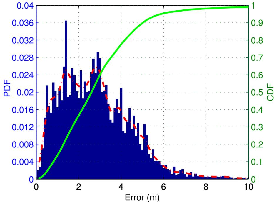
Figure 6.9: Histogram of error magnitudes collected over 1000 tests using the **VER** data set. Dotted line shows PDF estimate and solid line shows cumulative distribution function estimate.
