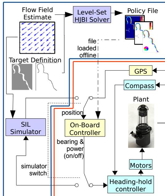
Figure 3.1: Controller Implementation Diagram – Orange box indicates online operations; Blue box indicates offline processes.
