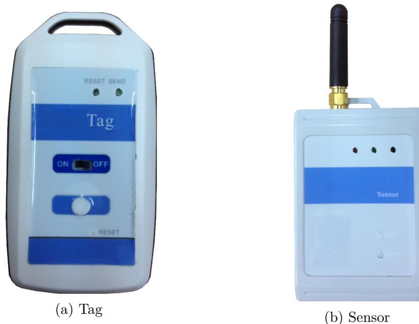
Figure 6.4: Active RFID devices used by the IPS sensor network.
