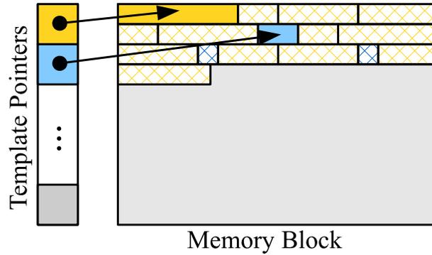
Figure 4.3: Diagram of the recordstore data structure in a typical scenario. There are two sets of records in this scenario, designated by the yellow and blue blocks. The solid yellow and blue blocks are the templates for that type of record and the hatched blocks are delta records which refer to the respective templates.
