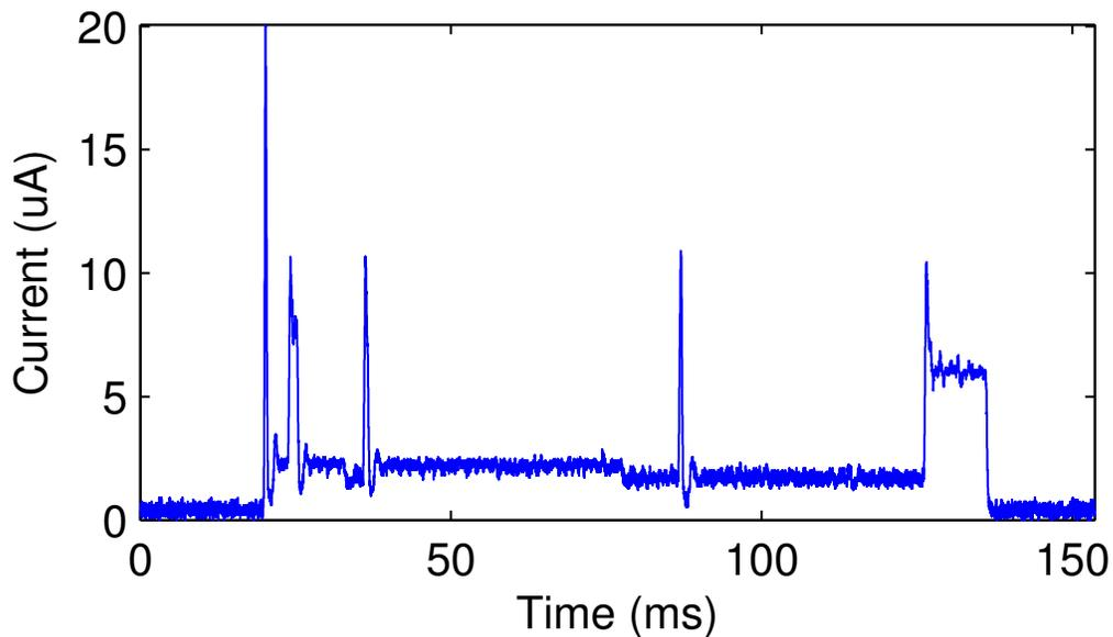
Figure 4.14: Current consumption while one environmental sample is being measured. In this example, 85 pAh was drained from the battery (excluding standby current).
