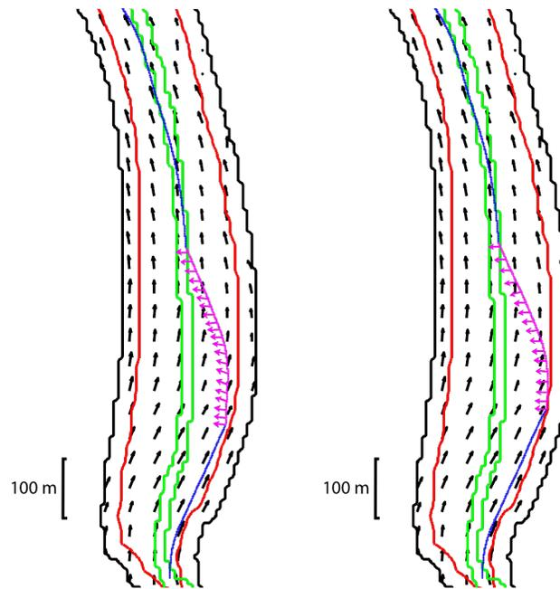
Figure 3.7: Simulated Trajectories with presence or absence of REALM flow field estimate. Left: known estimate. Right: no estimate incorporated.
