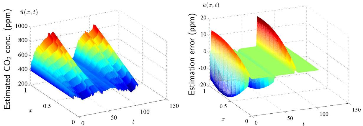
Figure 5.20: Left: The estimation of the CO<sub>2</sub> concentration  $\hat{u}(x, t)$  in the room for Experiment I. Right: The estimation error  $\tilde{u}(x, t) = u(x, t) - \hat{u}(x, t)$  of the CO<sub>2</sub> concentration in the room for Experiment I (shown after  $1 \times 100$  sec for a better visualization).
