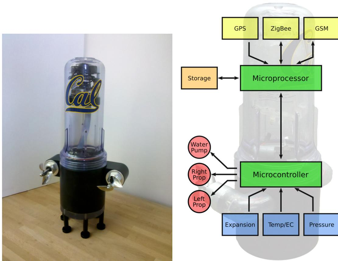
Figure 2.7: Left: motorized sensor unit. Right: modular breakdown of drifter.
