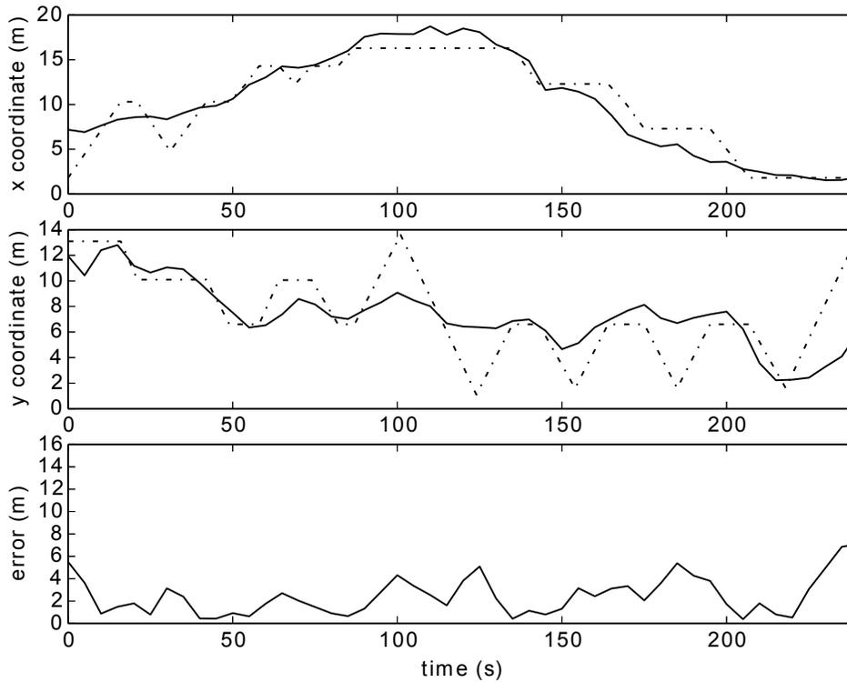
Figure 6.10: Example trajectory using default parameter values and **VER** data set. Dotted line is actual trajectory of occupant.
