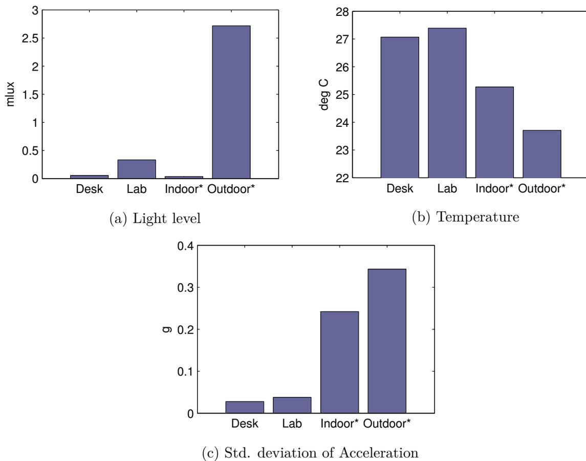
Figure 6.19: Features measured by the environmental sensing watch in different scenarios. \*The indoor and outdoor tests were measured while occupant was walking normally.
