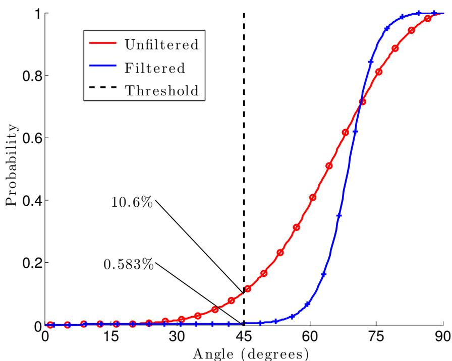
Figure 2.5: CDF of the angle calculated from the unfiltered (red circles) and filtered (blue pluses) accelerometer signal recorded by the Android phone. Unit was floating upright for the entirety of the 14 hour test. Black line shows the threshold value on which the software decides if the GPS position is valid.
