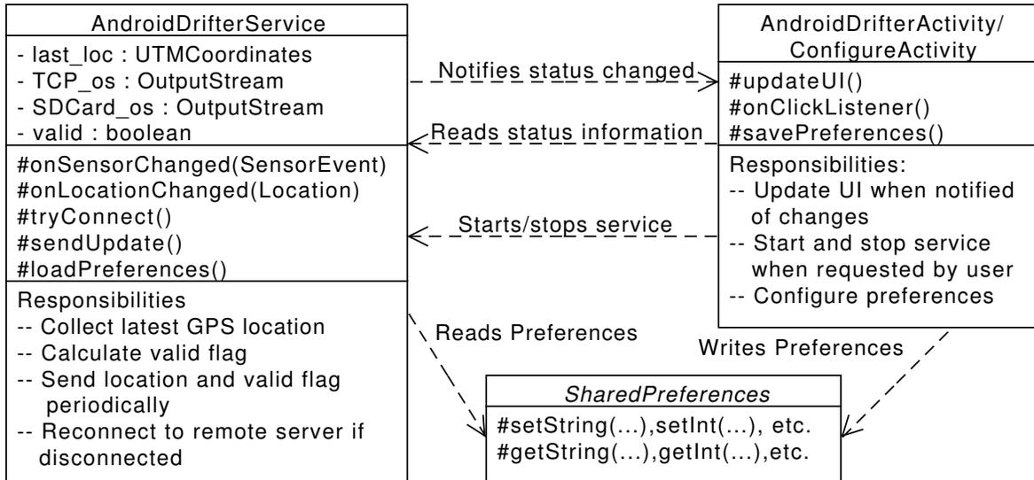
Figure 2.4: Simplified UML diagram showing interactions between software components of the Android drifter.
