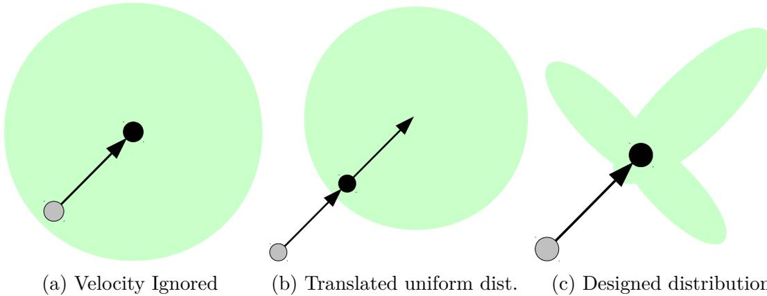
Figure 6.17: Transition distribution strategies given occupant velocity. Previous position is shown by a grey circle, current position is shown by a black circle, and the depiction of the transition distribution (i.e. where an occupant can move to) is shown in green.
