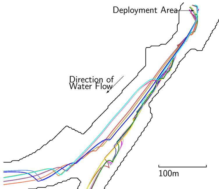
Figure 3.8: Trajectories of 20 simulated drifters performing path selection in Walnut Grove, CA. Drifters were deployed in a 20m diameter circle.
