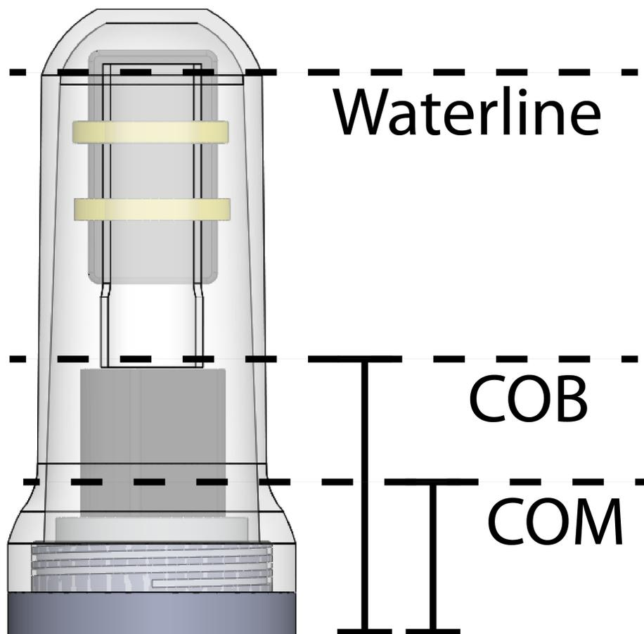
Figure 2.2: Sensor dimensions and COM and COB locations.
