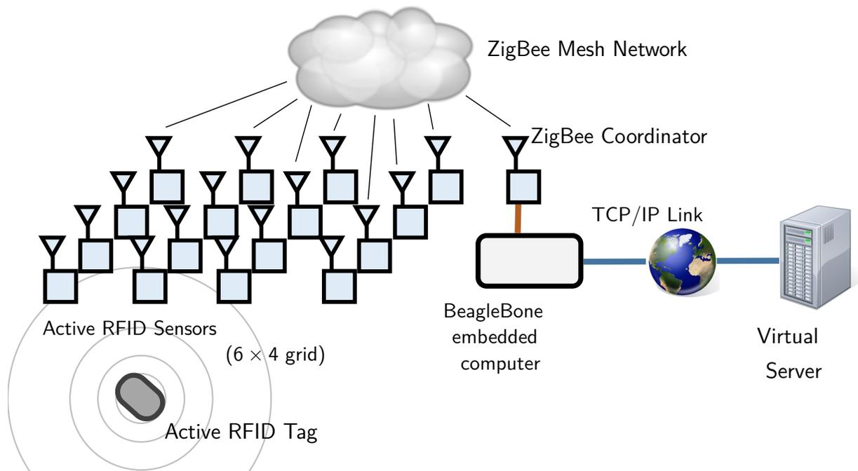
Figure 6.5: Network diagram showing data flow from beacons emitted by occupant-carried RFID tags to an Internet server which stores the data and runs the positioning program.
