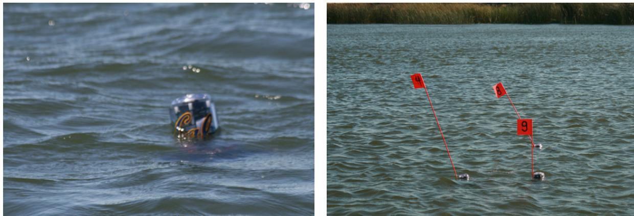
Figure 3.9: Left: drifter under motor power. Right: several drifters participating in experiment.
