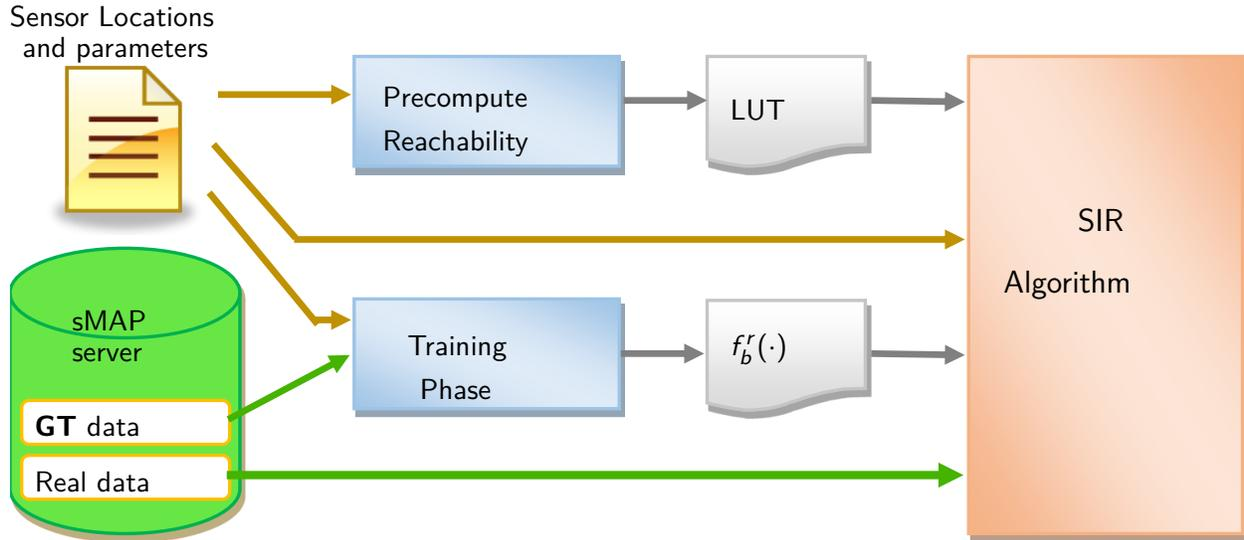
Figure 6.6: Process of the IPS software flow. Blue processes are precomputation steps, and grey files are intermediate outputs, but can be reused as long as parameters are held constant.
