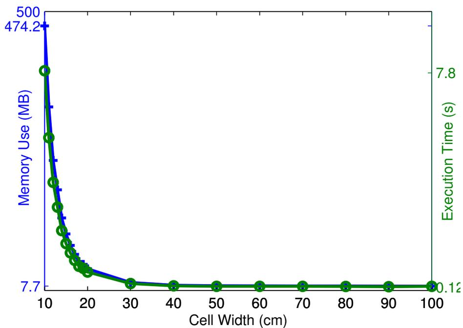
Figure 6.14: Plot of the resources used as a function of the reachability LUT cell width,  $C$ . Memory usage given by + markers and execution time given by  $\circ$  markers.
