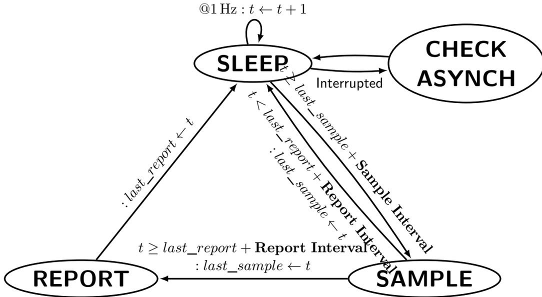
Figure 4.7: State machine diagram of the firmware running on the ATmega microcontroller of the environmental sensor. The variables  $t$ ,  $last\_sample$ , and  $last\_report$  represent time variables and initialized to 0. **Sample Interval** and **Report Interval** are configuration variables.
