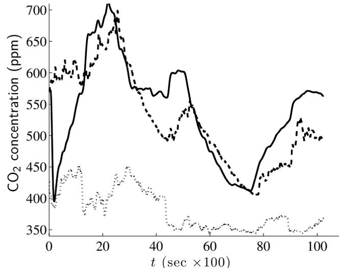
Figure 5.18: Solid line: The simulated concentration of the  $\text{CO}_2$  at the air return  $u(1, t)$  given by the model (5.1)–(5.4) for Experiment II. Dashed line: The concentration of the  $\text{CO}_2$  at the air return measured by the  $\text{CO}_2$  sensor. Dotted line: The concentration of  $\text{CO}_2$  at the air supply measured by the  $\text{CO}_2$  sensor.
