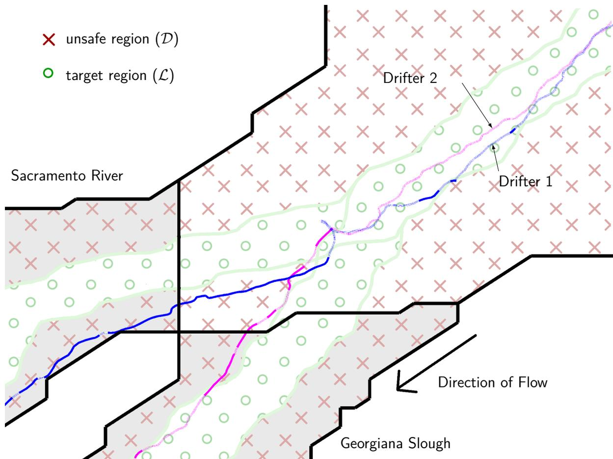
Figure 3.11: GPS Trajectories of two drifters performing the path-selection algorithm during a field test in Walnut Grove, CA. One of the drifters, shown by the blue trace, is tasked with proceeding down the Sacramento River, while the other drifter, in magenta, is tasked with proceeding down the Georgiana Slough. Along the trajectory, the faded segments indicate passive motion where the motors are off.
