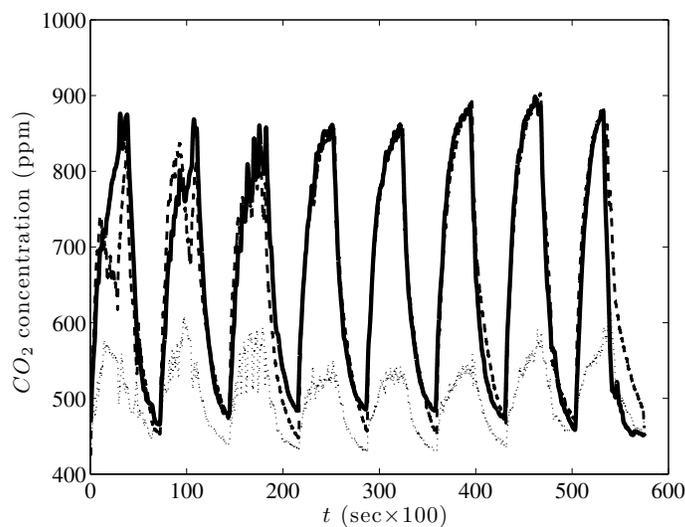
Figure 5.16: Solid line: The simulated concentration of  $\text{CO}_2$  at the air return  $u(1, t)$  given by the model (5.1)–(5.4) for Experiment I. Dashed line: The concentration of the  $\text{CO}_2$  at the air return measured by the  $\text{CO}_2$  sensor. Dotted line: The concentration of  $\text{CO}_2$  at the air supply measured by the  $\text{CO}_2$  sensor.
