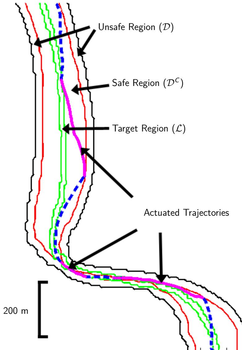
Figure 3.10: Drifter GPS Trajectory during northward tidal flow. The red line is a contour of  $V_{\text{shore}}$  and denotes the edge of the unsafe region. The green line is a contour of  $V_{\text{center}}$  and define the target region. Along the drifter trajectory, dotted lines indicate unactuated motion.
