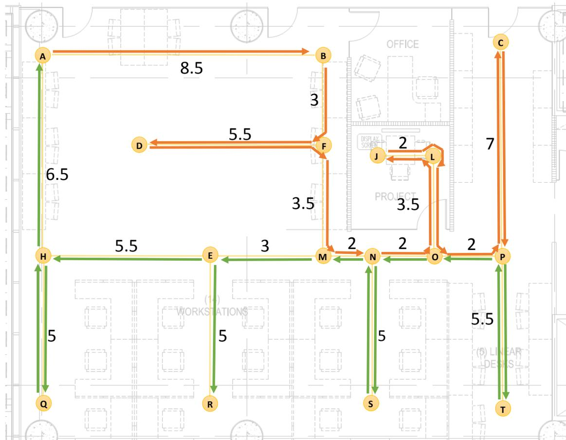
Figure 6.7: Ground truth trajectory diagram plotted over the floor plan of the office space. Trajectory starts at anchor point A and all distances are in meters.
