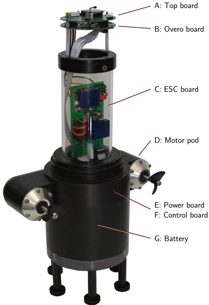
Figure 2.8: Generation 3 Drifter Hardware Components.
