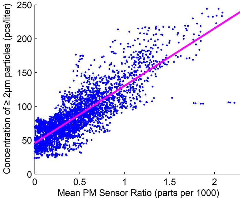
Figure 5.8: Scatter plot of  $\geq 2 \mu\text{m}$  particle concentration from OPC against  $\geq 2.5 \mu\text{m}$  output from the DSM501A.
