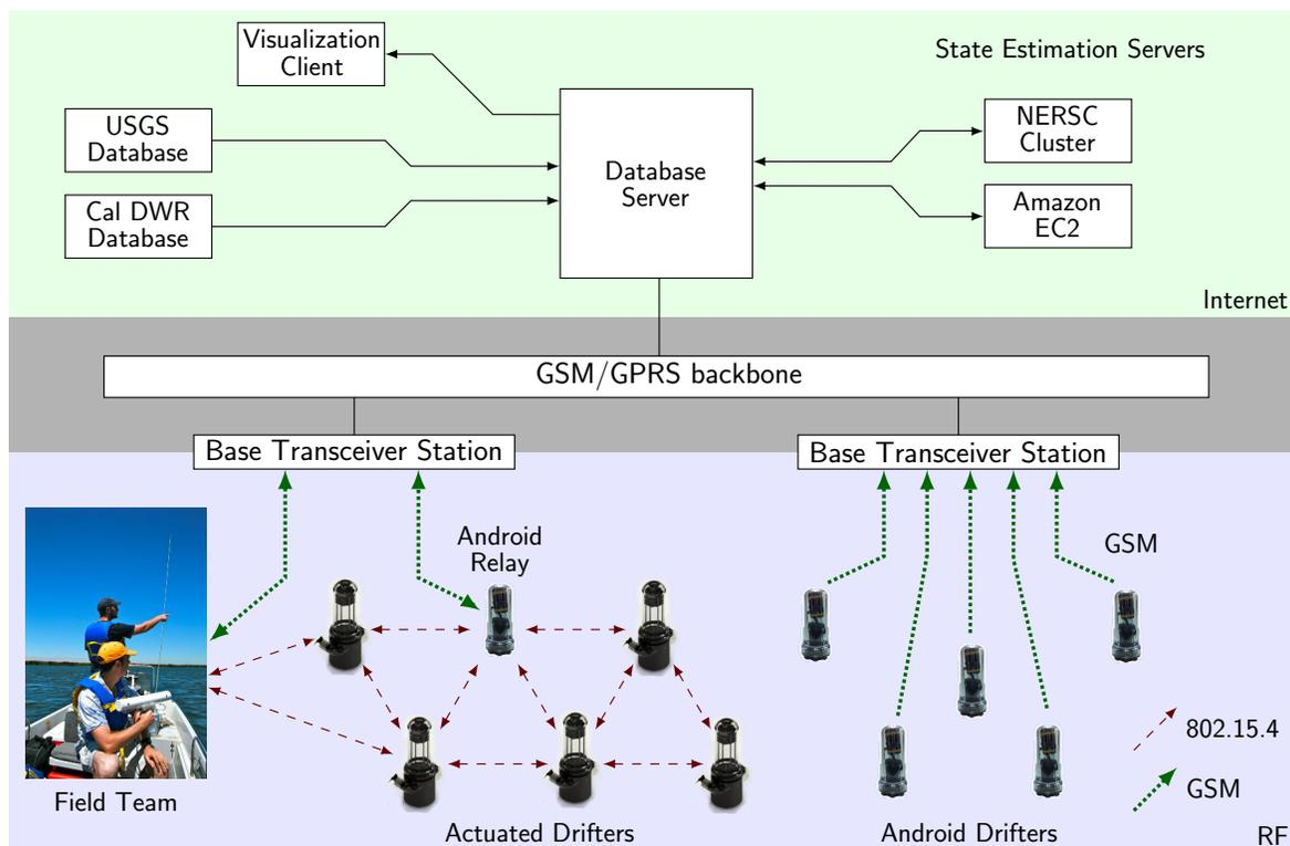
Figure 2.10: Communication architecture, showing the flow of data from drifters in the field to the database server and computation servers via the GSM service.
