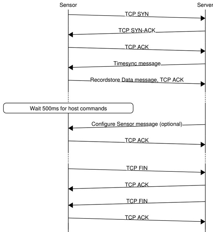
Figure 4.4: Typical exchange between sensor and server during one report, showing packets at the transport layer and above.
