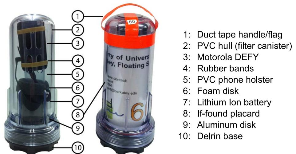
Figure 5. Android drifter set for the study with complete parts list.
