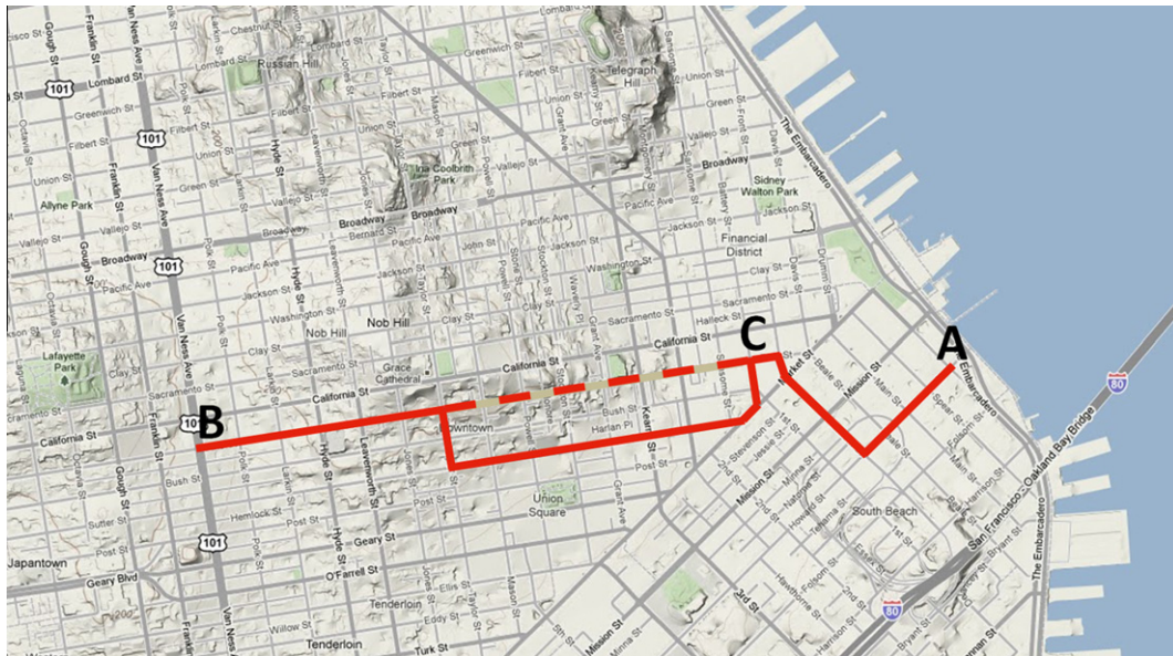
Fig. 9. Commute from point A to point B: two drivers depart from point A at 8:50 pm on February 1st with a budget of 20 min to reach point B. They are routed by the SOTA module. Because their realized travel times differ, their recommended routes differ. The first driver is suggested to turn left at point C, whereas the second driver is suggested to drive straight.
