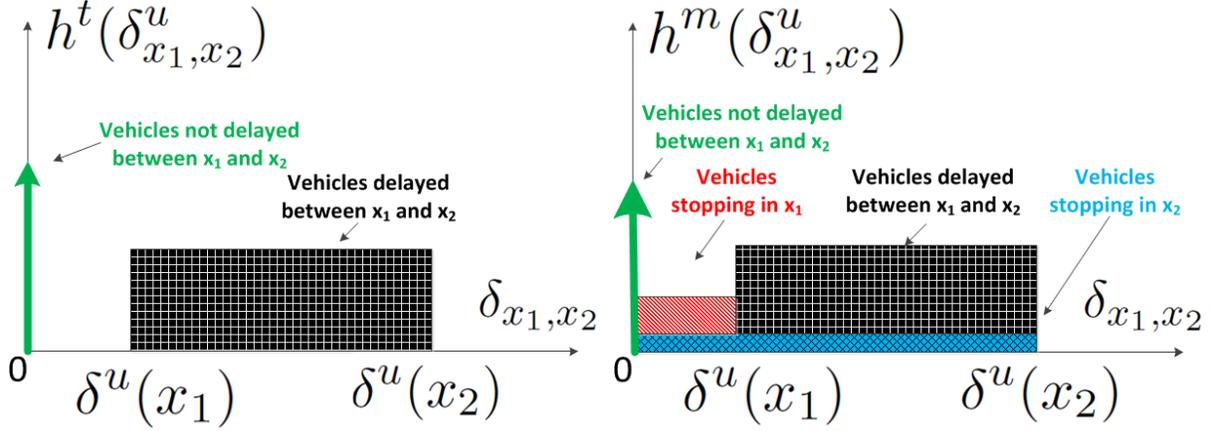
Figure 6: **(Left)** Probability distribution of the total delay between  $x_1$  and  $x_2$  in the undersaturated regime. **(Right)** Probability distribution of the measured delay between  $x_1$  and  $x_2$  in the undersaturated regime. Vehicles are assumed to be sampled uniformly in time.
