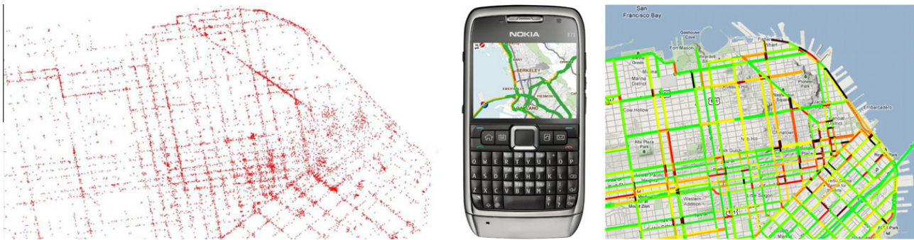
Fig. 1. Mobile Millennium system, Left: cumulated raw probe vehicle data collected on a typical day, for one of the feeds of Mobile Millennium. Each dot corresponds to a point where a probe vehicle emitted its position data. Center: traffic monitoring system output displayed on a phone. Right: web interface of real time monitoring system.
