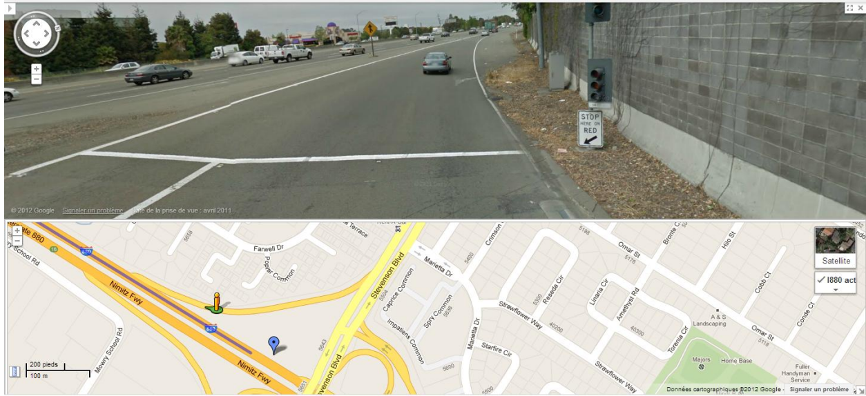
On-ramp and metered light at detector 1
