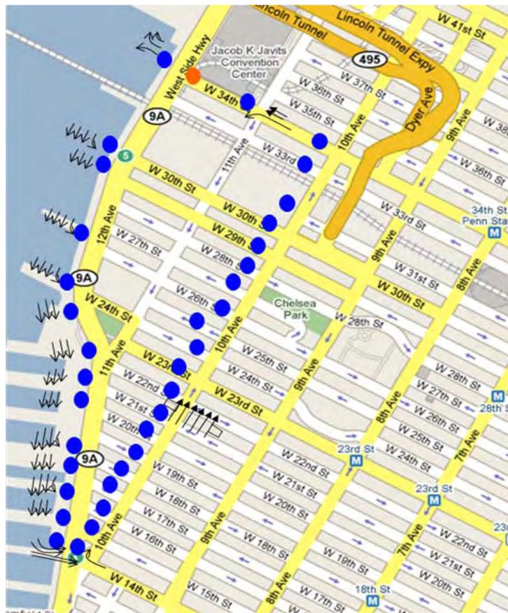
Figure 2.14. Map of NYC arterial route used for each NYC road test and the ITS World Congress demonstration. The red dot indicates the traffic signal nearest to the Javits Convention Center.
