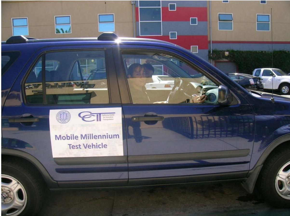
**Figure 1.1.** A Mobile Millennium test vehicle ready for field test deployment in Berkeley, CA. Note that the vehicle includes a driver and an observer (passenger) responsible for recording traffic information along the route.
