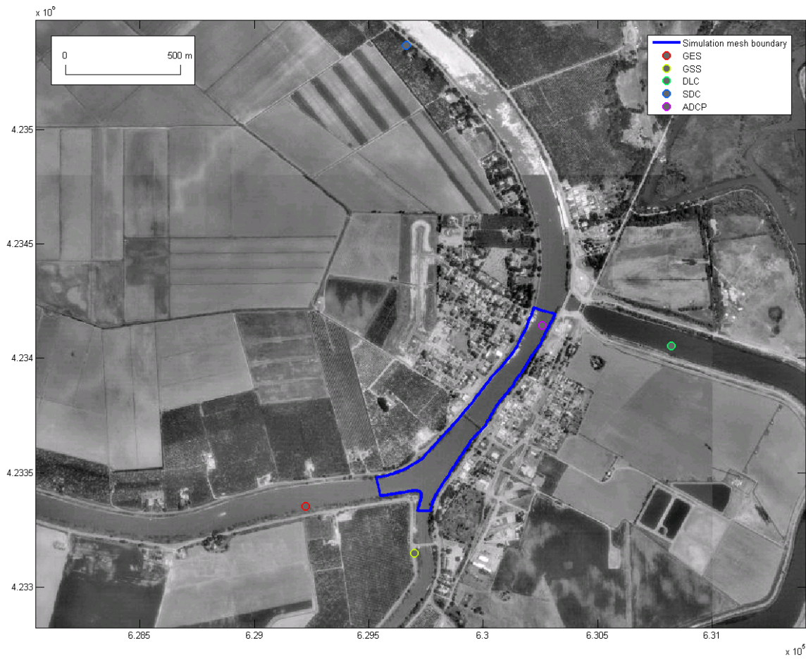
Figure 2.19: Satellite image of the portion of the Sacramento River studied, located near the town of Walnut Grove. The location of the ADCP sensor is represented by a blue dot in the top right part of the domain. Figure courtesy of Andrew Tinka.
