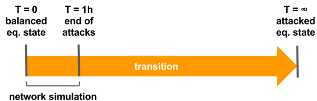
Fig. 3. Steady-state analysis gives re-balancing and attack strategies for the balanced and attacked equilibrium states respectively ( T = 0 and T = \infty ). Since the attacked equilibrium state is not attainable in practice, a network simulation evaluates losses after 1h of attacks.
