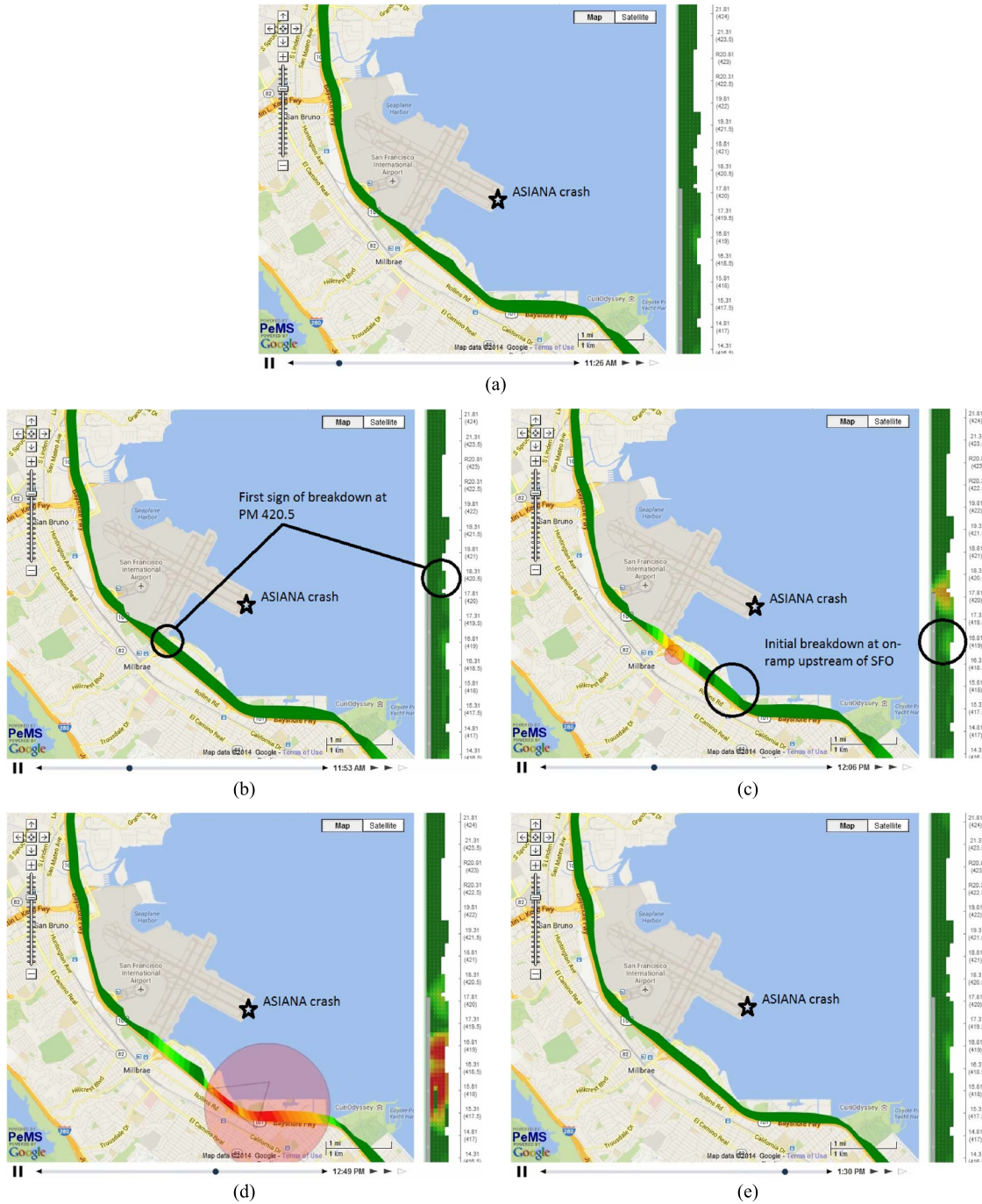
Fig. 17. Traffic situation on the US101N at different times on July 6th, 2013. Two breakdowns can be observed: the first at 11:53 am, the second at 12:10 pm.
