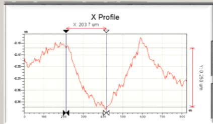
600 um membrane defelction, PRESSURE ON
