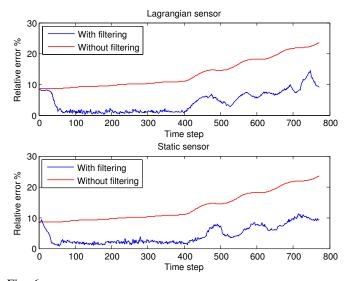
Fig. 6: The time evolution of the relative error of the estimated velocity while using a Lagrangian sensor (top), and an Eulerian sensor (bottom).
