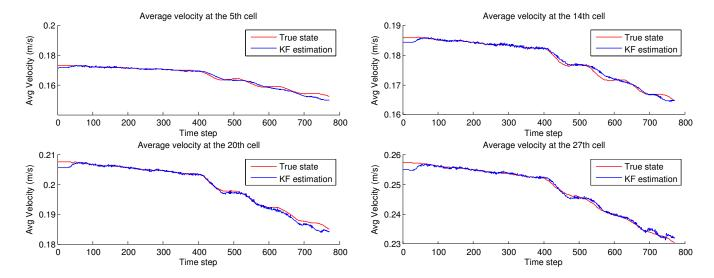
Fig. 5: The time evolution of the estimated velocity and the true velocity at four cells.
