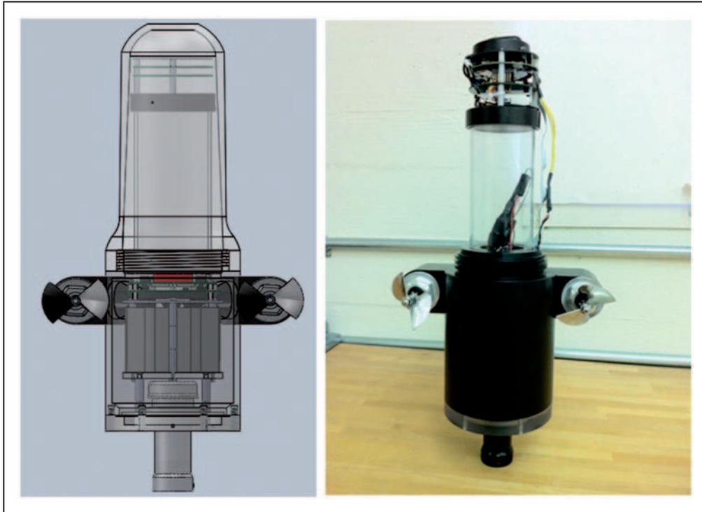
**Figure 24.** Floating sensor modified for single-beam depth finder.
