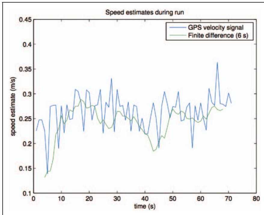
Figure 14. Vehicle velocity inferred from GPS signal.
