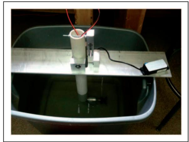
**Figure 12.** Motor force test platform: submerged motor unit is attached to an extended arm which pivots against a force transducer. Power is applied to the motor at a range of values and output force is recorded in Matlab.
