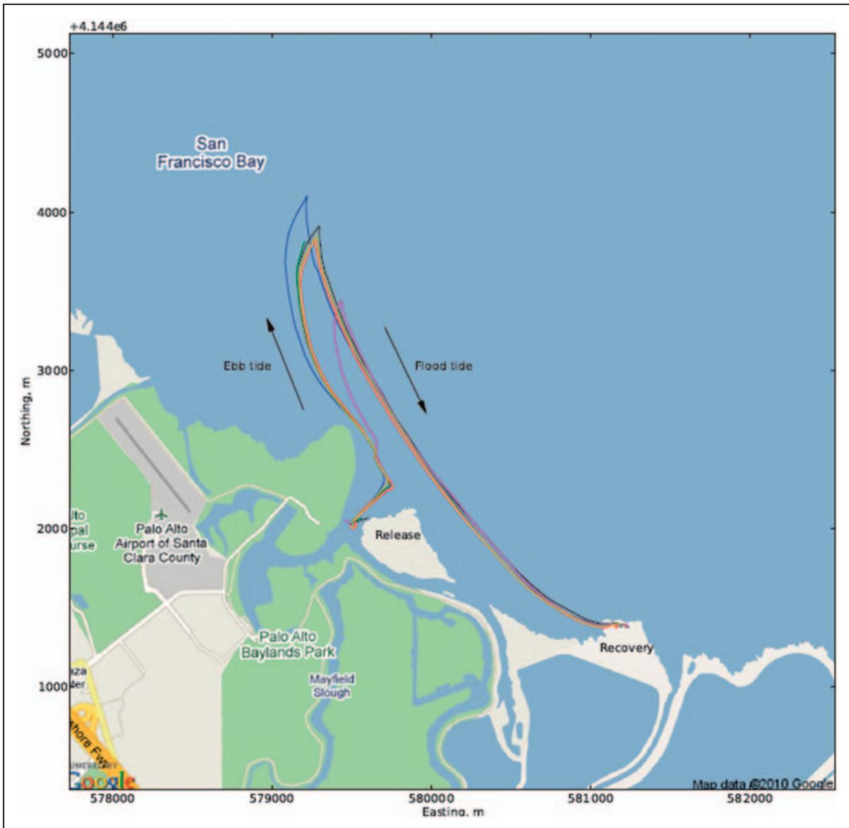
Figure 23. GPS traces from floating sensors during 24-h San Francisco Bay experiment.
