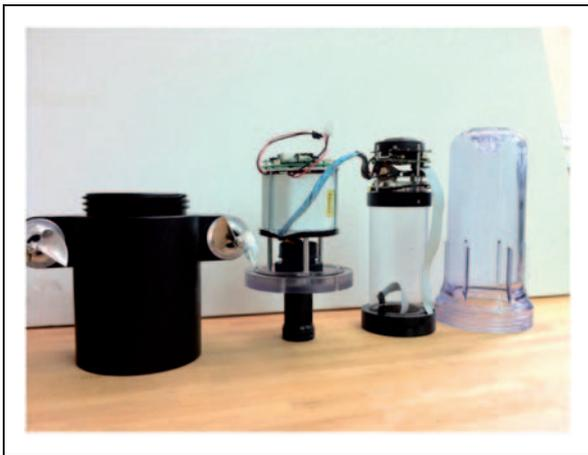
**Figure 7.** Modular structure of vehicle's internals: (from left to right) Delrin lower hull with removable motor pods, lower electronics assembly with battery and sensors, upper electronics assembly with microprocessors and guidance/location sensors, and clear PVC upper hull.
