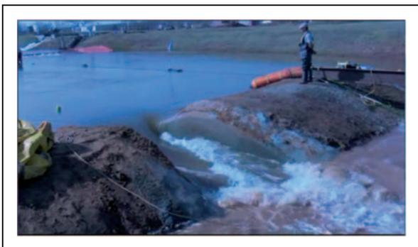
Figure 19. Floating sensor about to pass through the breach.
