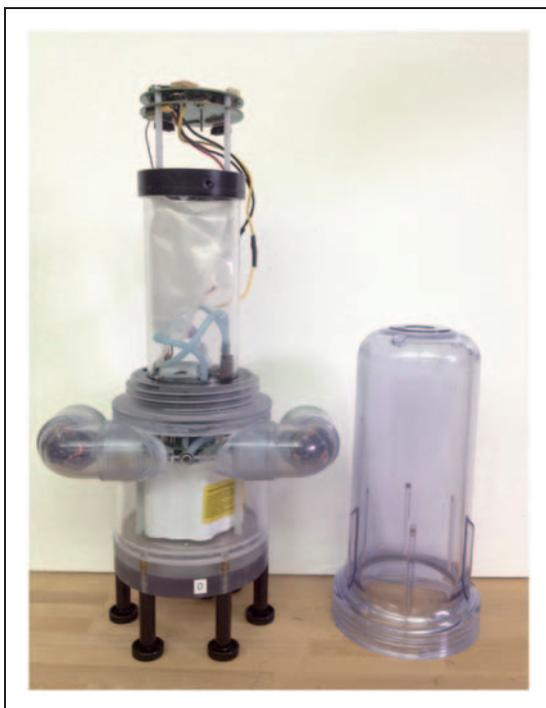
**Figure 16.** Prototype sensor with buoyancy control.
