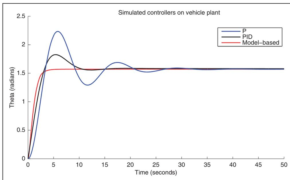
**Figure 11.** Simulink simulation of the effect of three proposed controllers on the vehicle plant.
