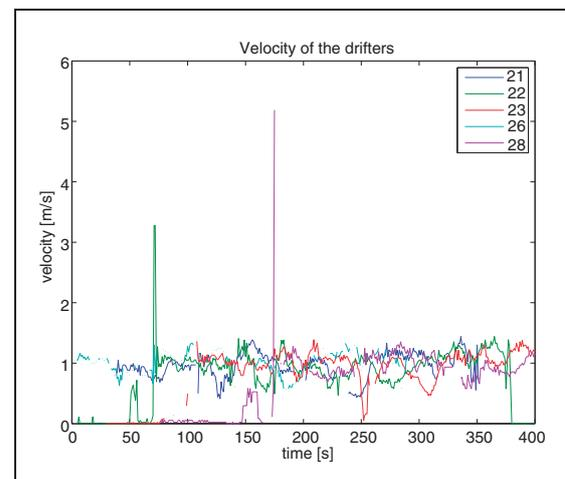
Figure 21. Measured sensor velocity during canal deployment.<sup>13</sup>
