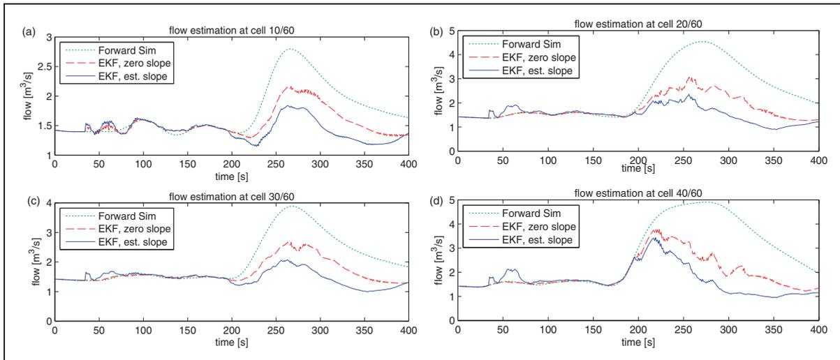
Figure 22. Estimated flow in discretized “cells” of the canal.<sup>13</sup>
