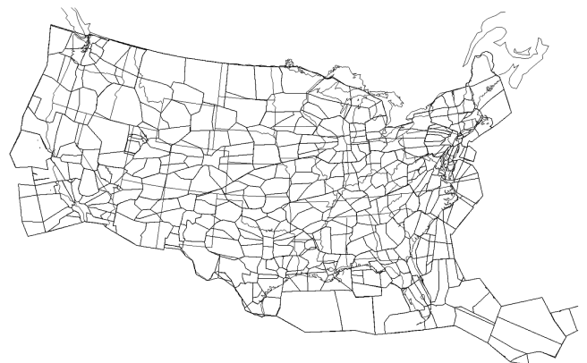
Fig. 1 Map of airspace considered in this study; 20 continental ARTCCs including 284 high-altitude sectors in the United States. Figure obtained using FACET [10].
