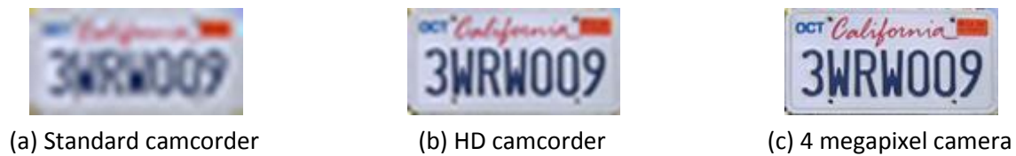
Figure 7.2: Simulated resolution for three camera types, assuming one camera per lane.
