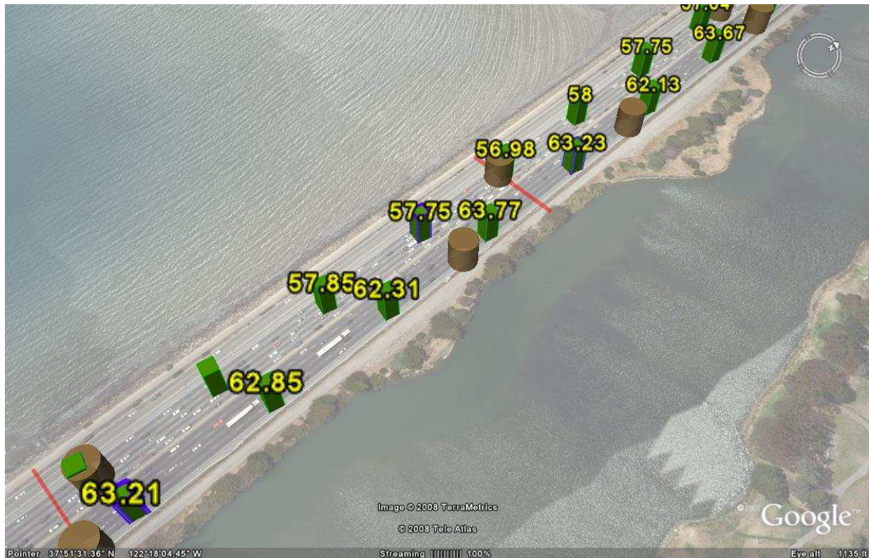
Figure 4.5: Satellite image of the first experiment site I-80 near Berkeley, CA. The red lines represent the locations of the VTLs, the blue squares show the speed recorded by the VTL, and the green squares represent the position and speed stored in the phone log. The brown circles represent the readings from the vehicle speedometer.
