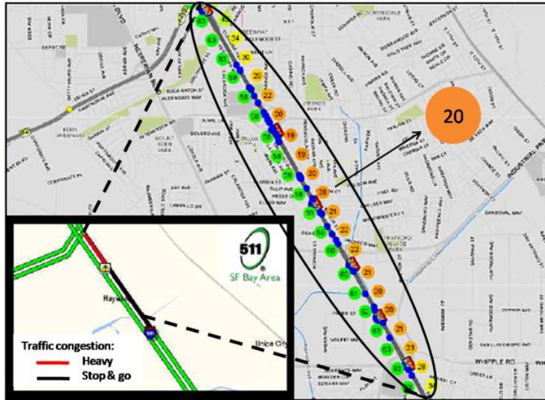
Figure 9.1: Snapshot of the live traffic feed provided by the system in the present work (and from 511.org in the inset) at 10:52am on February 8, 2008. Traffic conditions after an incident on the northbound direction of I-880 are displayed. Numbers in circles correspond to speed in mph.
