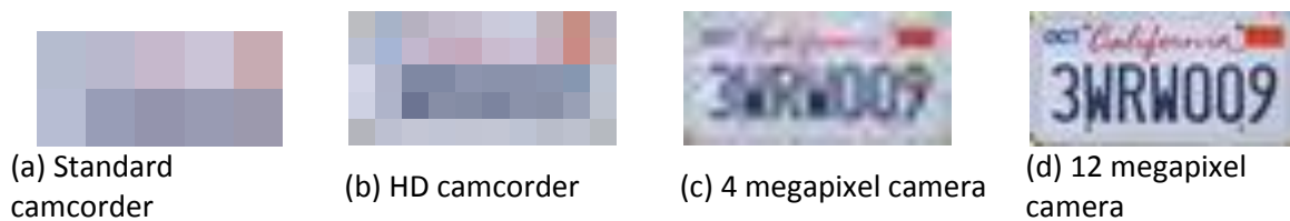
Figure 7.3: Simulated resolution for four camera types, assuming one camera for five lanes.
