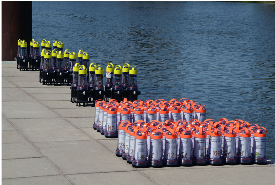
Figure 1. Drifter fleet on the Walnut Grove Public Dock on May 9, 2012, prior to deployment. In the background, with yellow tops, are actuated drifters, described in Section 2.1; in the foreground, with orange tops, are passive drifters, described in Section 2.2. Photo credit: Jérôme Thai.
