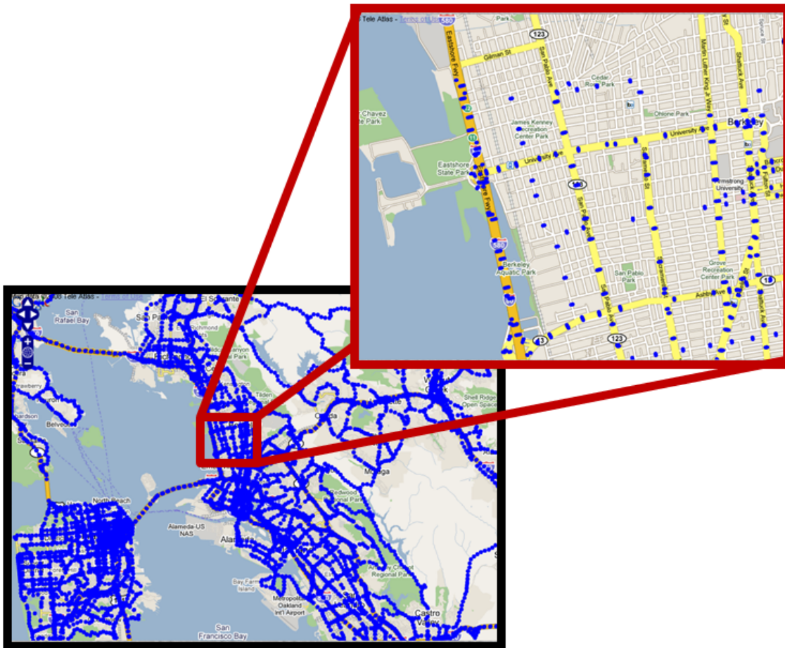
Figure 2.1: Example of a Bay Area VTL deployment as part of the Mobile Millennium system.
