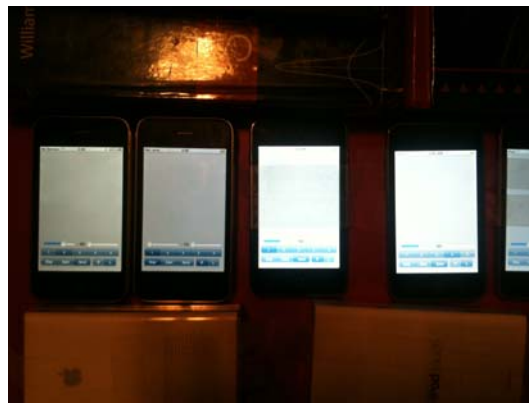
FIG. 13. A photograph of testing setup, with Loosely connected and rigidly connected iPhones on the same shaking surface
