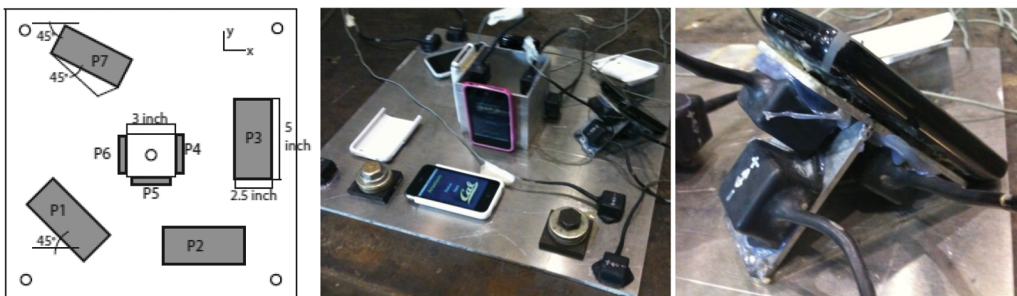
Figure 1. Phone and instrumentation set up during the shake table tests.
