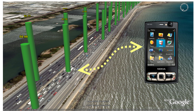
Fig. 1. Mobile Century -Traffic Monitoring using GPS Phones. The Nokia N95 mobile device is used to collect and transmit anonymous speed and position data when on-board vehicles. The height of the columns correspond to the speed of a vehicle equipped with an N95 on I-80 near Berkeley, CA.
