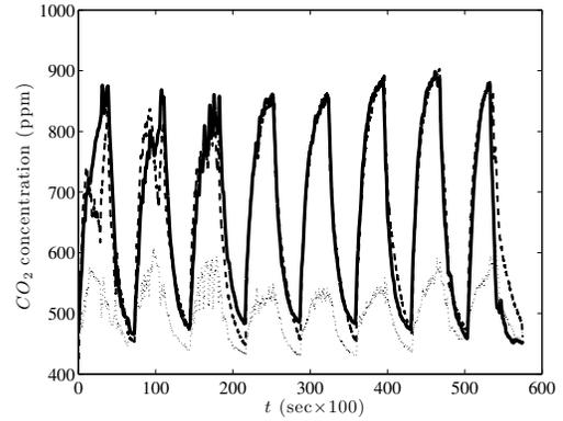
Fig. 5. Solid: The simulated concentration of CO<sub>2</sub> at the air return  $u(1, t)$  given by the model (1)–(4) for Experiment I. Dashed: The concentration of the CO<sub>2</sub> at the air return measured by the CO<sub>2</sub> sensor. Dotted: The concentration of CO<sub>2</sub> at the air supply measured by the CO<sub>2</sub> sensor.
