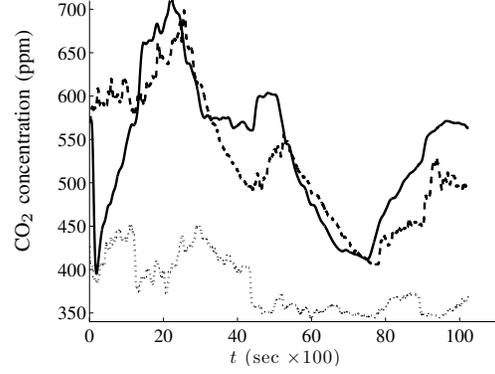
Fig. 7. Solid: The simulated concentration of the  $CO_2$  at the air return  $u(1, t)$  given by the model (1)–(4) for Experiment II. Dashed: The concentration of the  $CO_2$  at the air return measured by the  $CO_2$  sensor. Dotted: The concentration of  $CO_2$  at the air supply measured by the  $CO_2$  sensor.
