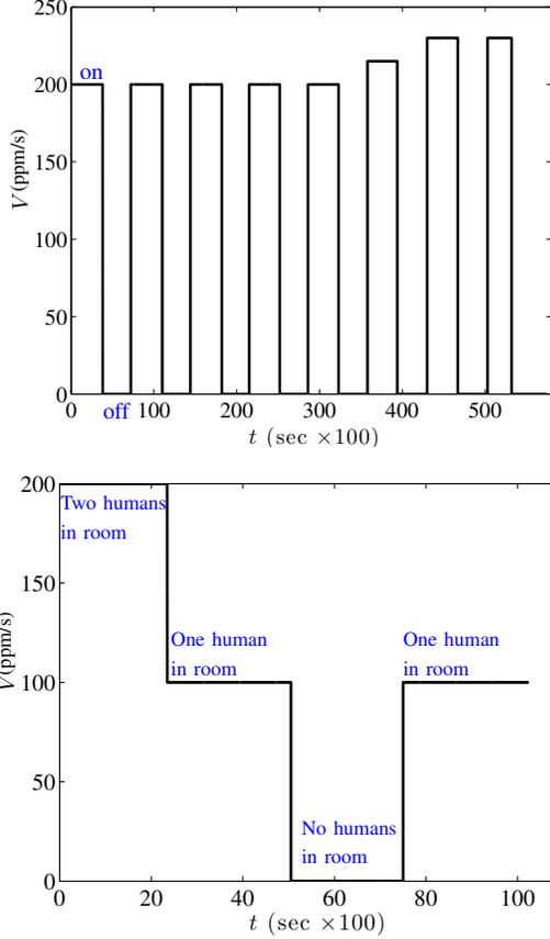
Fig. 6. Top: The input  $V$  to the model (1)–(4) from Experiment I modeling the concentration of  $CO_2$  that is released from the pump. When  $V = 0$  the  $CO_2$  pump is turned off and when  $V \neq 0$  the  $CO_2$  pump is turned on. Bottom: The input  $V$  to the model (1)–(4) from Experiment II modeling the input concentration of  $CO_2$  from the humans.
