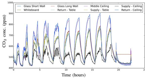
Fig. 2. CO<sub>2</sub> concentrations during Experiment I. Showing measurements from all 7 locations over the approximately 22 hour experiment.
