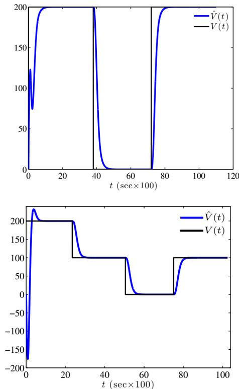
Fig. 8. Top: Estimation  $\hat{V}$  (blue line) of the pump input  $V$  (black line) in Fig. 6 for Experiment I. Bottom: The estimation  $\hat{V}$  (blue line) of the input  $V$  (black line) in Fig. 6 produced from the people for Experiment II.
