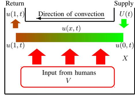
Fig. 4. Geometrical representation of our model. Fresh air ( $U$ ) enters the room from the supply vent. Air near the ceiling ( $u$ ) convects from the air supply to the air return. Humans produce CO<sub>2</sub> ( $V$ ) rising ( $X$ ) to the ceiling.
