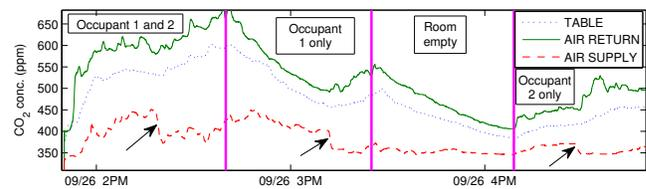
Fig. 3. CO<sub>2</sub> concentrations during Experiment II. Showing measurements from 3 locations in the conference room over 3 hour experiment. Magenta lines indicate when occupancy changes occurred. The arrows indicate the time instants at which the ventilation rate increases<sup>2</sup>.
