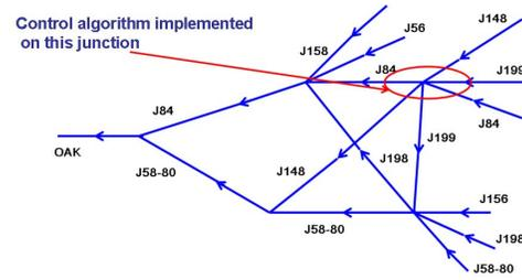
Fig. 2. Network used for the optimisation containing 16 links and 5 junctions. This is an idealised figure representing the portion of the airspace considered, and links are not drawn to scale. The links are numbered according to the jetways they represent. We will focus on the junction circled in red.
