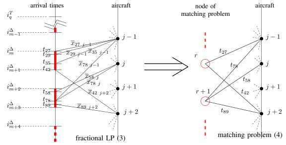
Fig. 2. Illustration of the procedure Matching. This procedure transforms the feasible fractional solution  $\overline{x}_{ij}$  into a weighted matching problem. In the fractional LP solution, only the nonzero  $\overline{x}_{ij}$  are represented (solid if they are in the range of the figure, dashed if they connect aircraft with arrival times outside the figure). On the right plot, the weights are the arrival times from the fractional LP solution: for example,  $\Theta_{rj-1} = t_{27}$ .
