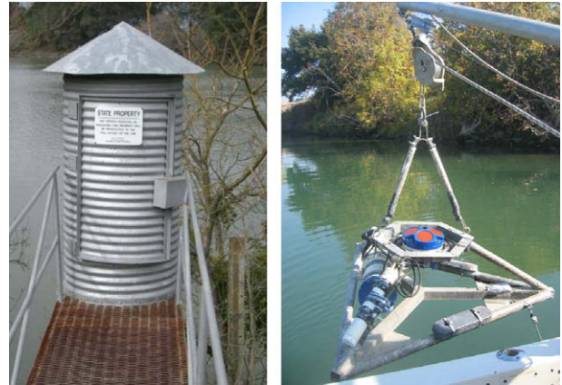
Fig. 7. (Left) USGS sensor station at GSS, used as a measurement sensor. (Right) Deployable ADCP sensor, used in Section 3.5 for gathering the validation data (three of them were deployed between 11/01/2007 and 11/12/2007 in order to gather the data for this study).
