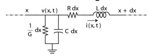
Combining KVL and KCL and eliminating the current yields the telegraph equation:
