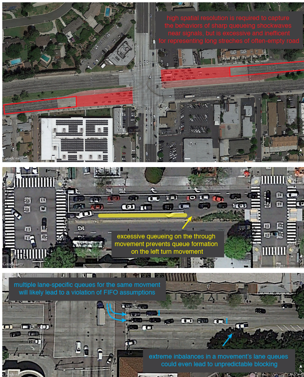
Figure 1.3: Many aspects of the queuing dynamics observed on signalized roadways make accurate modeling difficult. Sharp queueing shockwaves on signalized roadways would require excessive spatial discretization for accurate representation via CTM. Furthermore, a basic CTM is unable to model the interactions between movement-specific queues which form immediately upstream of a signalized intersection.
