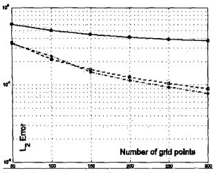
Fig. 1.  $L_2$  error due to the discretization method, as a function of the number of grid points for both schemes. The analytical solution presented in [3] is used for this comparison. Lax-Friedrichs scheme (solid), Jameson-Schmidt-Turkel scheme (-.), left-centered scheme (-.).
