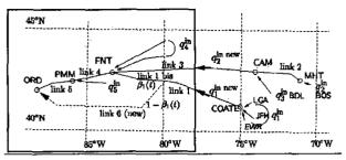
Fig. 2. Network model shown in [3]. We now add a divergence link in order to be able to show that we are able to control the density of aircraft by splitting the flow. For this simulation, we restrict ourselves to the box including ORD. The new additional link is shown with a dashed line. We call  $\beta_1$  the portion of flow which stays on link 1 (called 1 bis) and  $1 - \beta_1$  the portion which goes into the new link (link 6).
