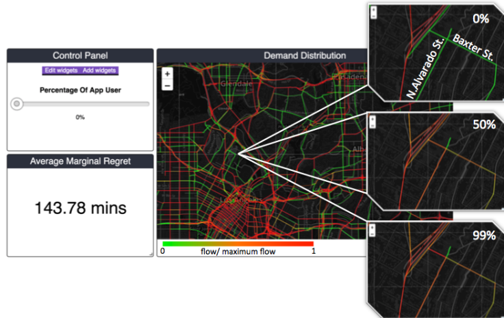
Fig. 2. The RIDER DSS Dashboard displaying the demand distribution across the LA Basin network, and the demand distribution on Baxter St. and N. Alvarado St. with 0, 50, and 99% app users (best viewed in color).
