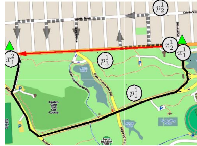
Fig. 5 Example of a failure case when using a Hidden Markov Model: the solid black path will be favored over all the other paths
