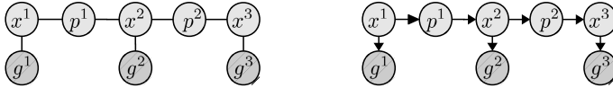
Fig. 4 Illustration of the graphical models used in the path inference filter (CRF, left), and commonly found in the literature (HMM, right), defined over a trajectory \tau = x^1 p^1 x^2 p^2 x^3 and a sequence of observations g^{1:3}
