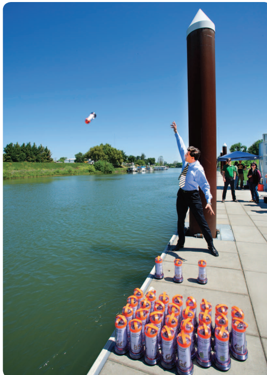
Alex Bayen throws one of the passive floating sensors in the Sacramento River in Walnut Grove, California.
