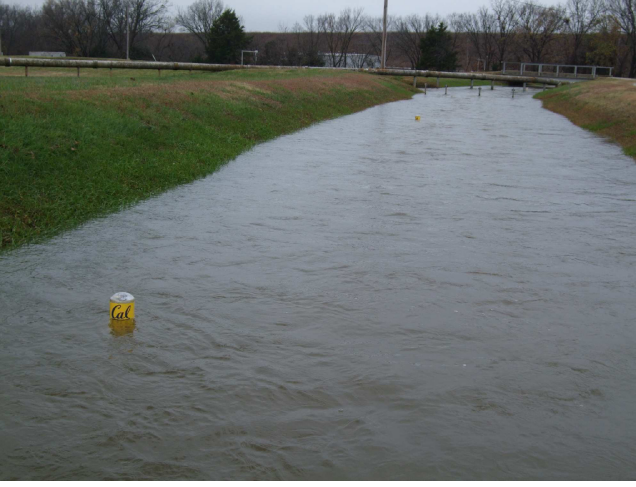
Fig. 10. Two drifters in the HERU facility supply canal.
